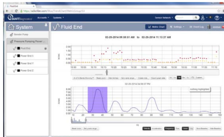
Machine Condition Monitoring Software Vibration Metric Chart
