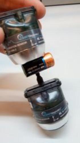
Figure 8 - Remove the Battery with A Second Sensor
