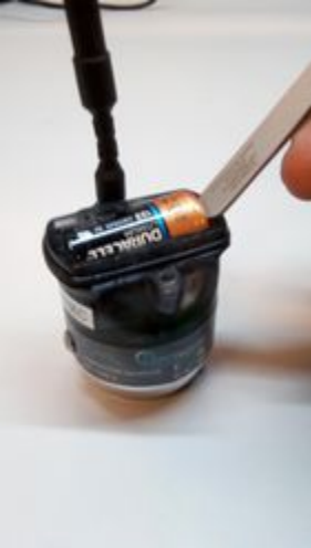
Figure 9 - Use the Back End of Tweezers if Necessary to Pry Battery Out of Sensor
