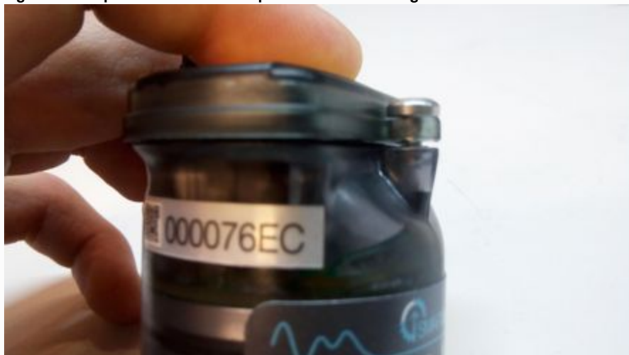
Figure 13 - Gap Between Sensor Cap and Sensor Housing
