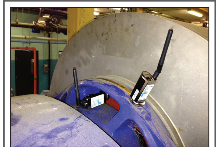
Top: The location of two SmartDiagnostics® vibration sensors on a dewatering centrifuge at a wastewater treatment plant. Bottom: A screen capture of the data coming from a dewatering centrifuge showing increasing vibration levels and potential failure.
