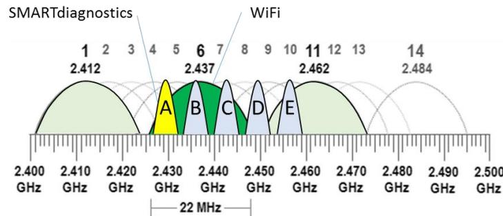
Notice that SmartDiagnostics® channel D does not overlap with primary WiFi® channels 1, 6, and 11, which allows them to coexist without interfering. In the case where WiFi® Channel 6 is used, SmartDiagnostics® channels D and E can be used. Similarly, if WiFi® channels 1 and 11 are used, SmartDiagnostics® channels A, B, C can be used without interfering.
