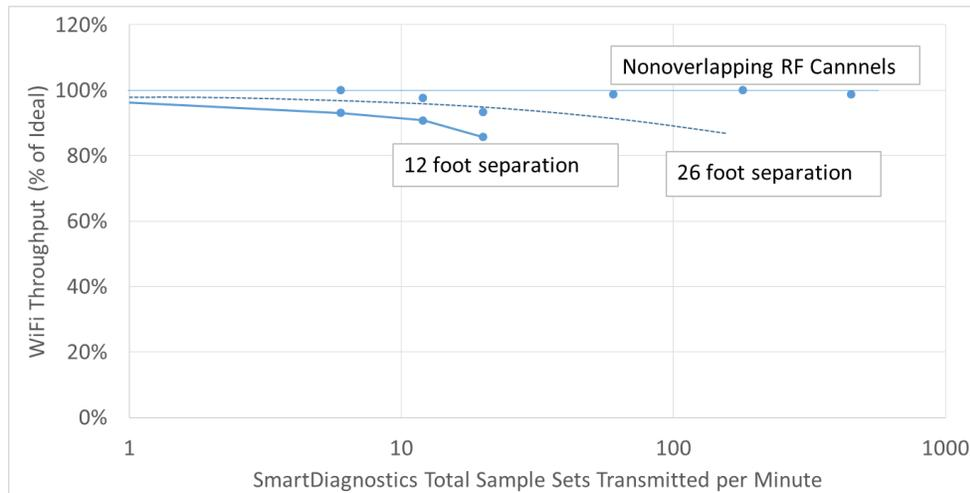
This assessment was made for a case where the separation distance between the WiFi® Access Point (transmitter location) was 12’ and 26’ away from the SmartDiagnostics® network. The horizontal axis shows SmartDiagnostics® total sample sets transmitted per minute, which can be roughly calculated as the number of sensors in a wireless coverage area divided by the average data set transmission interval (e.g., 650 sensors/30 minutes = 22 total sample sets transmitted per minute).
