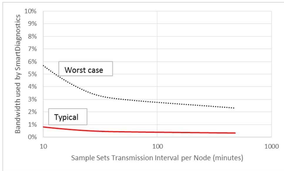
**The figure shows that 100 nodes transmitting large (1650 point) data sets every 30 minutes consumes between 0.5-3.4% of a single, narrow band, channel (only one of the 5 channels shown in the frequency spectrum).**
